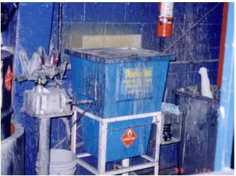
Figure 3-11. Spray Gun Cleaning System at Autobody Shop
