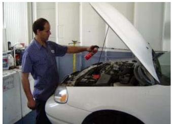
Figure 3-15. Technician Performing General Purpose Degreasing.
