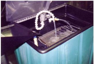
Figure 2-3. Immersion Parts Cleaner
