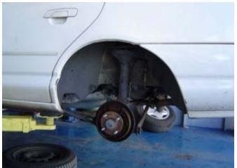
Figure 3-14. Vehicle with Drum Brakes.
