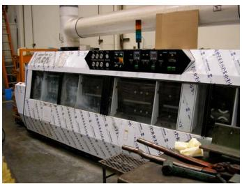
Figure 3-4. Conveyorized Water Board Cleaning System
