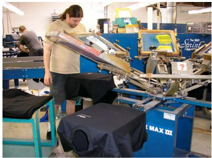
Figure 3-19. Automated Press for Textile Printing
